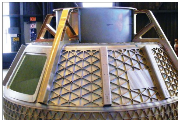
Pressure testing of the crew compartment structure anchors was conducted in September at the Bigelow Aerospace facility in Las Vegas.
